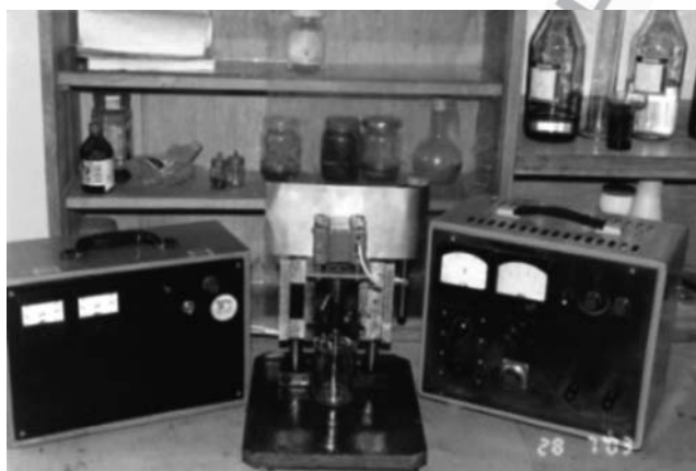
Fig. 11.2 The installation for synthesis of nanocarbon structures and Me-carbon composites in the liquid phase
